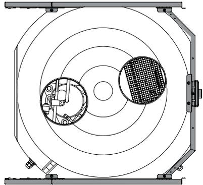
HPSW pump allows to change the position of the connectors. Connectors may be directed to the back or side of device (right or left side).
