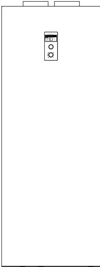
Connection to the water supply system must be done in accordance with the binding norms. Heating pump HPSW 2 is a pressure device adapted for connection to water supply system not exceeding pressure 0,6MPa. If the water pressure exceeds 0,6 MPa, install a pressure reducing valve in front of the machine.
